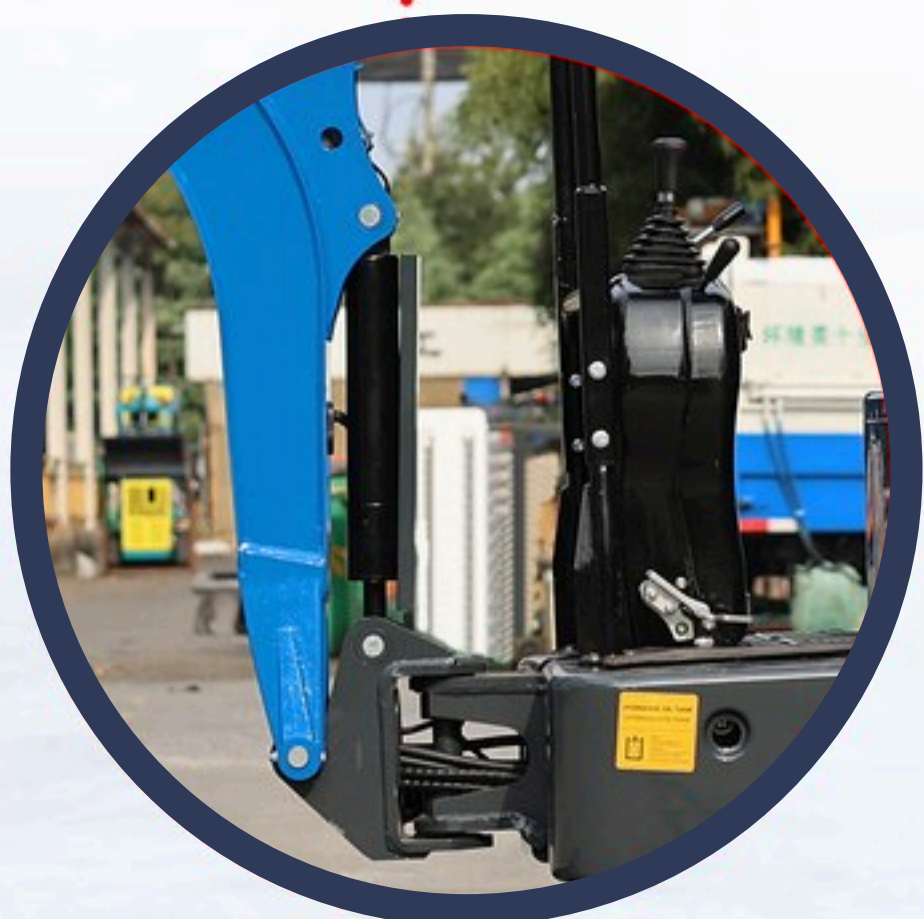
Top-mounted boom cylinder + cylinder guard plate
